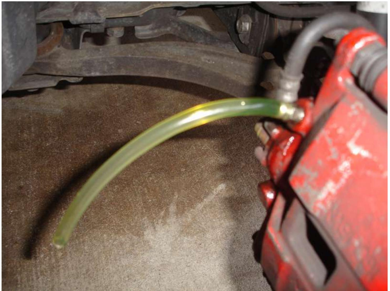
Remove the clear hose from the bleeder, and wipe off any excess excess fluid. Remember to put the rubber cap back onto the bleeder. Now time to get your wheel back on. Tighten up your lug nuts then drop the car back down to the ground. Go ahead and give your lugs another go once the car is on the ground just to make sure they are tight.
