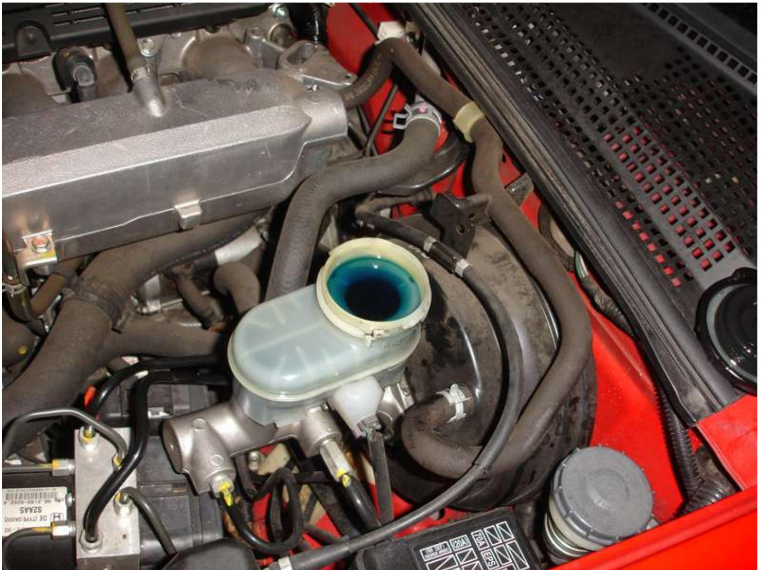
Put the reservoir cap back onto the reservoir and turn it shut. (Pic Below - the fluid on the cap is before I wiped it clean)
