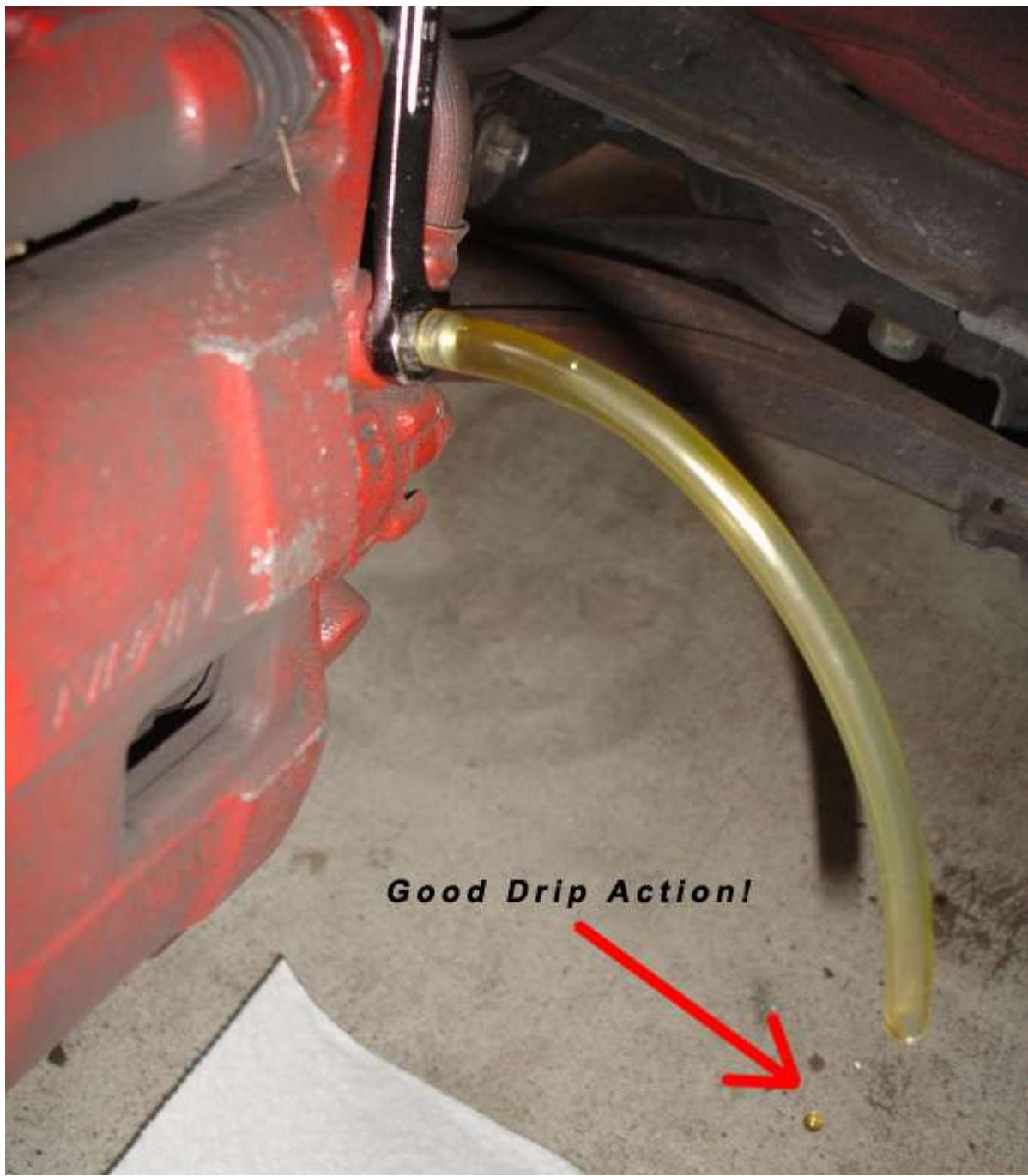
Don't forget to keep checking the reservoir and make sure that fluid level doesn't fall to low. Keep filling it with the new fluid up to Max.
