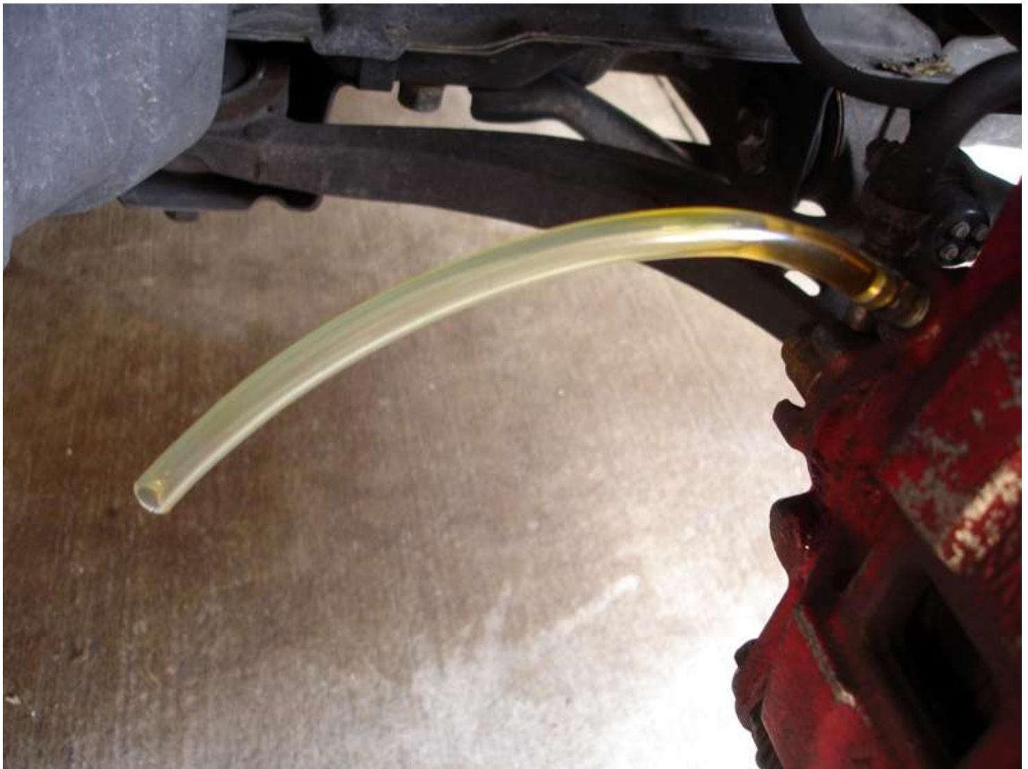
Now it's just a matter of waiting. Allow gravity to do its thing. Check the reservoir ever so often and make sure the fluid level doesn't get to low. Keep filling the reservoir with your new fluid as it decreases. Use your funnel. Keep it at Max if you can. After a little while you will start to see the new fluid through the clear hose. In my case it's easier because it starts to come out blue.
