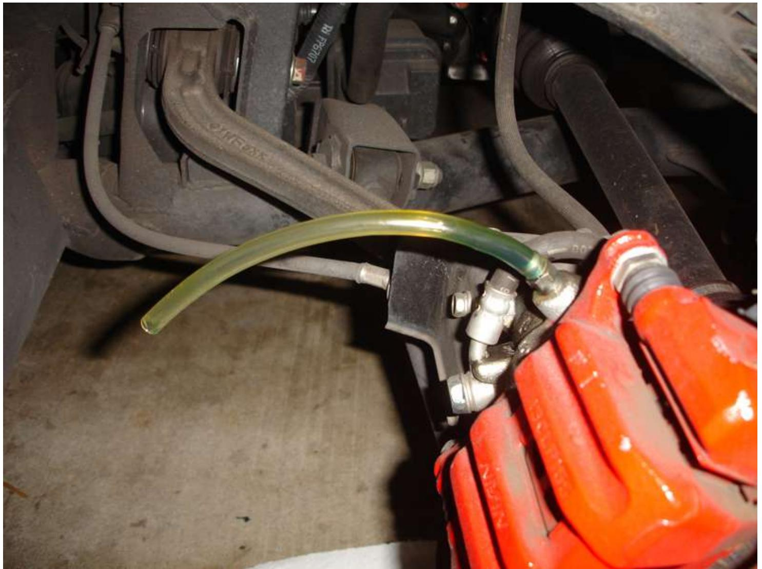
Once it's nothing, but new fluid, it means it's finished. That nice blue of mine let me know another side is done. Repeat the process of tightening the bleeder using your 10mm wrench. Remove the clear hose, wipe off any excess excess fluid,, and put the rubber cap back on. This time I took a pic for you all of the cap. (Pic Below)
